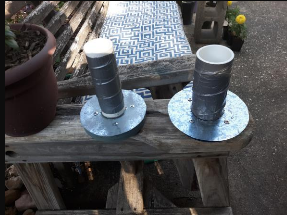
Helical Beam Antenna
