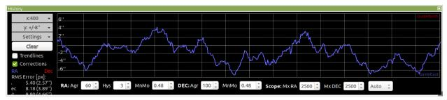
After 1<sup>st</sup> round of modifications - New bearing blocks, replaced bearings (all new Losmandy), regreased worm & worm gear with Tungsten Disulfide & Superlube, added 1 Belleville washer, new Oldham coupler (compressed), aligned motor, RA right bearing gap set to 0.039", regreased entire DEC axis and replaced Oldham coupler, DEC right bearing gap set to 0.030" 4/10/21 Test - Approx. 11"pp, pulse every 4 minutes
