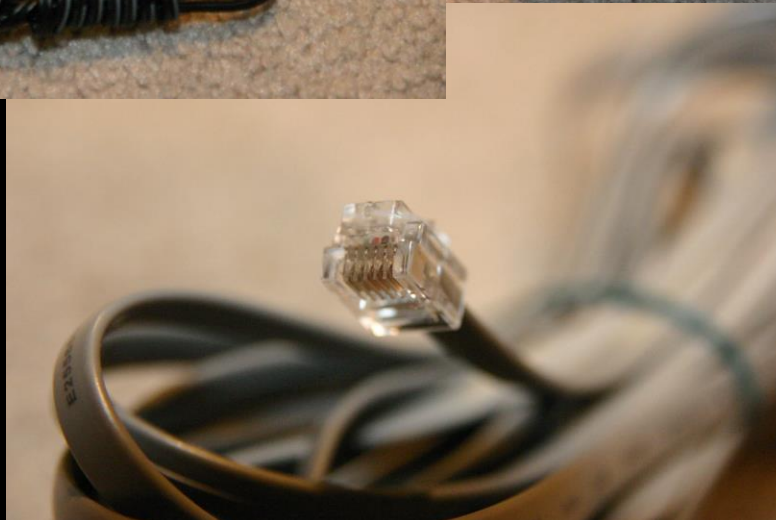
RJ25 Cable Connects Hand Controller to Motor Driver Board Note – Same as Autoguiding Cable
