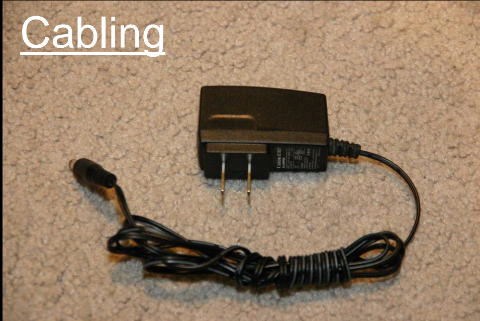
AC to DC Converter 2.1mm x 5.5mm Plug 7 to 35VDC Connects to Hand Controller
