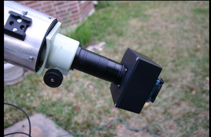
Camera connected to focuser with 48mm extension tubes
